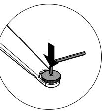
**EN** If desks are to be used for longer periods of time. The knurled screws must be tightened fully with an Inbus key.
